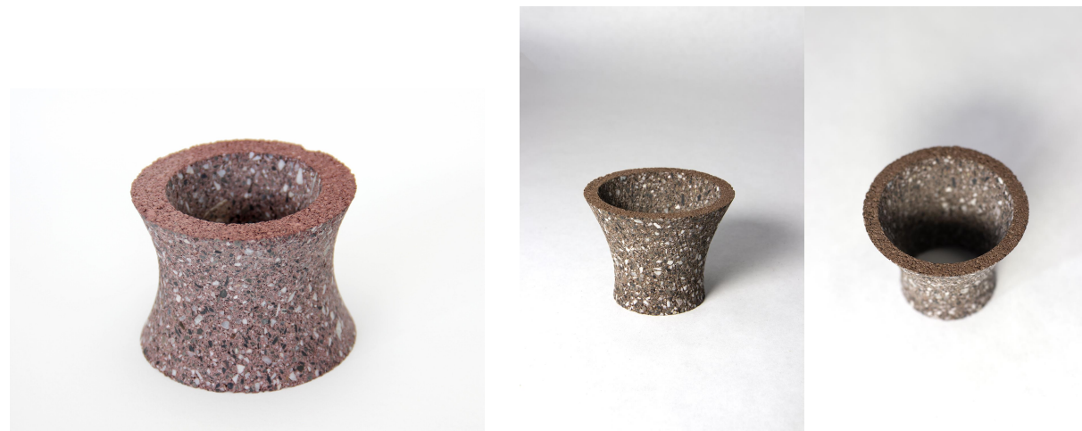
Figure 1. Hyperboloids waterjet cut from standard masonry brick. Images by the authors.
