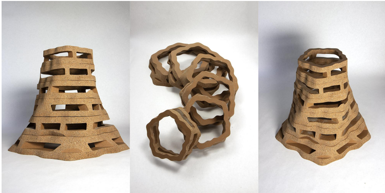
Figure 3. Tapering sections with 5-point rotational symmetry waterjet cut from terra cotta. Images by the authors.
