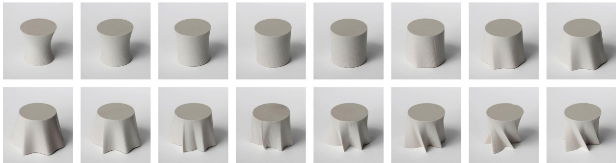
Figure 4. Sequence of rotational swarf cuts. Multi-axis waterjet movements were programmed from the same parametric model. Images by the authors.
